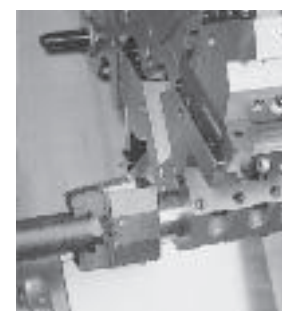
Powerpull on turret pulling bar into position
